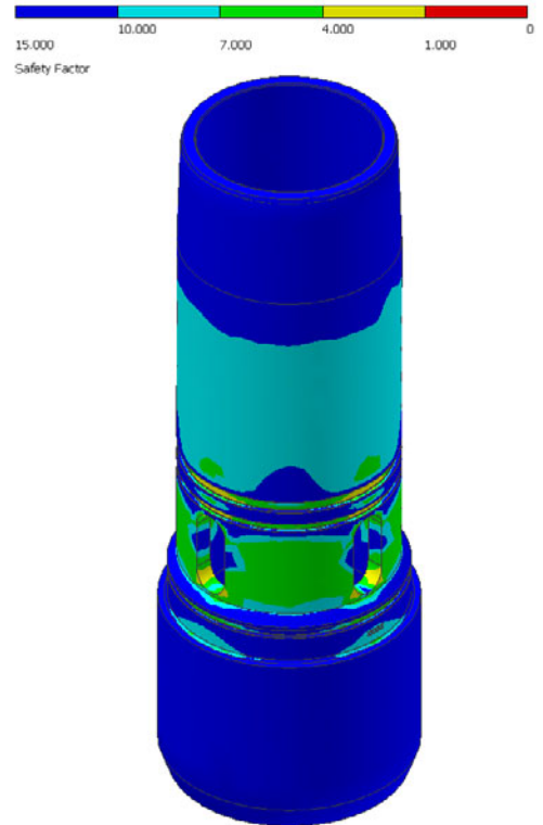
Figure 6.5 4-1/2: Safety Factor at 4930 ft-lb Cooler colours indicate higher safety factor. Red areas indicate yielding.
