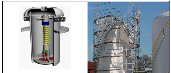
Left: Cut away of the recessed housing and internals of the Anti-freeze Thief Hatch.
