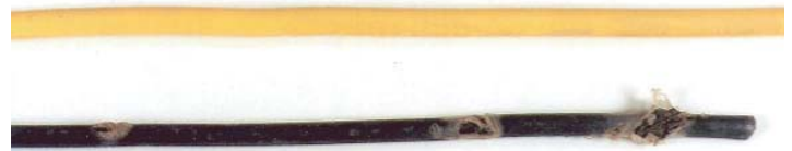
Above: Copper Clad Steel tracer wire cross-section. Below: HDPE Jacket wire (yellow) vs. THHN jacket wire (black) from same installation.
