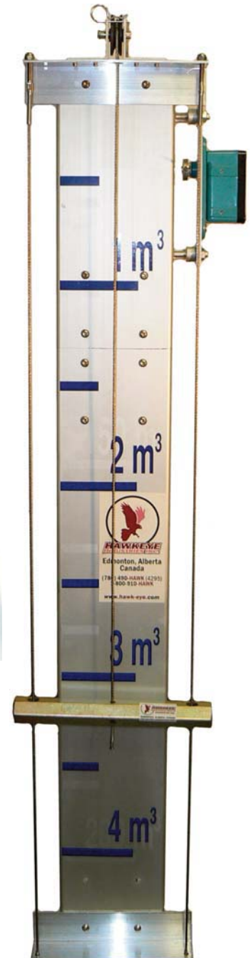
Above right: Gauge board top brack with indicator guides and idler pulley.
