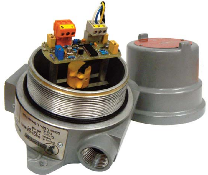
Above: Goshawk Transmitter with cover removed
